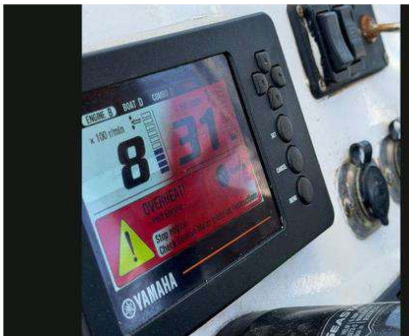
Figura 4. Alarma OVERHEAT Port Engine activa en el Command Link Plus. RPM motor babor: 800, motor estribor: 3.100.
